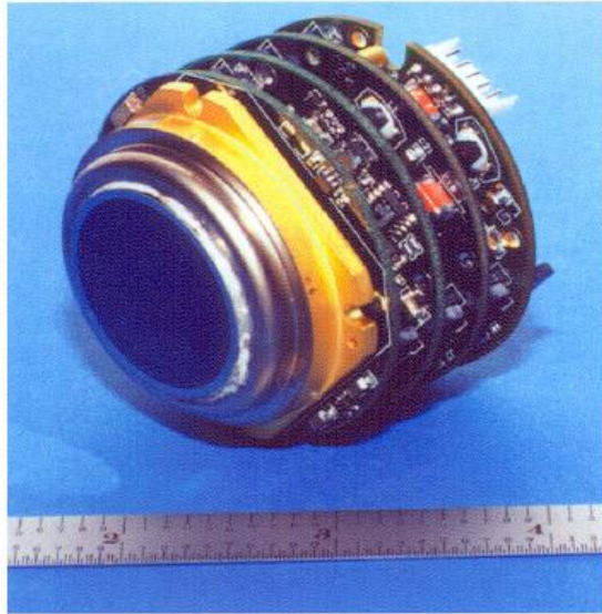
Figure 1 Microbolometer Sensor Engine for EVS
